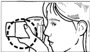
Note: As the focal length becomes larger, shaking the camera becomes more noticeable. Hold the camera firmly with both hands while keeping elbows at sides to prevent the camera from shaking.
