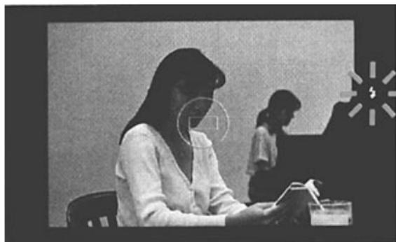
Note: If you press the shutter release button with
