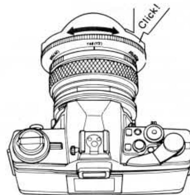
After switching the built-in filters, be sure to refocus the lens.
