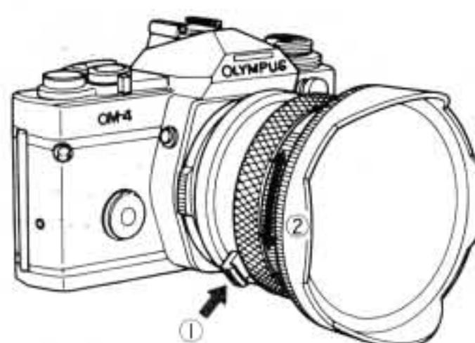
The viewfinder shows correct exposure indications, only when the lens is not shifted.
